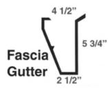
Our most popular model. Its deep back design with built-in drip edge allows it to be used with or without fascia board.
